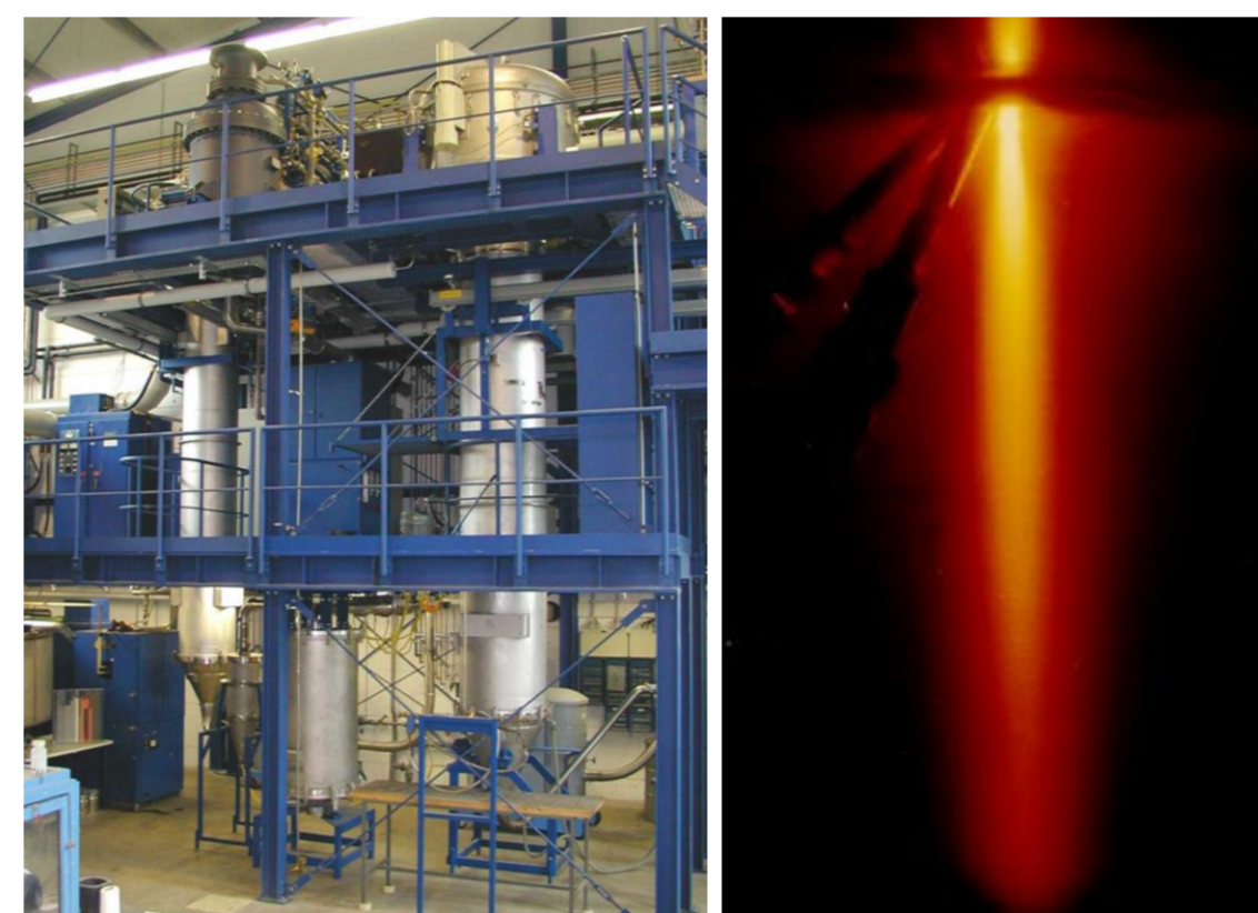
Atomizing towers (left) and atomized molten metal jet (right) for the manufacturing of spherical metal powders at UMSICHT.
