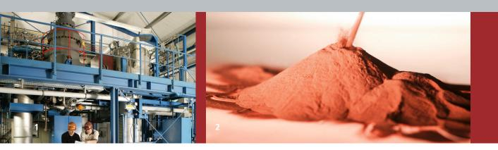
In-house engineered plants for melt atomization with hot gas up to 1000 °C at 25 bar atomizing gas pressure.
