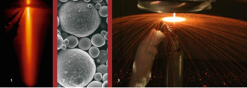
Fine powders through high pressure and hot gas atomization.
